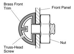
Figure 5 - Attaching Brass Front Trim to Front Panel
